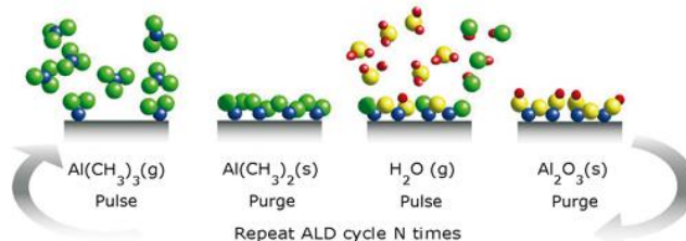
Figure 1. Schematic of an ALD cycle: example of \text{Al}_2\text{O}_3 deposition from \text{Al}(\text{CH}_3)_3 and \text{H}_2\text{O} . Step 1: pulse of the reactant 1, \text{Al}(\text{CH}_3)_3 , leading to its absorption on the surface. Step 2: purge of the unreacted precursor and of the by-products. Step 3: pulse of the reactant 2, \text{H}_2\text{O} , which reacts with the surface species created by precursor 1. Step 4: purge of the unreacted precursor 2 and of the by-products. Taken from ref 5
